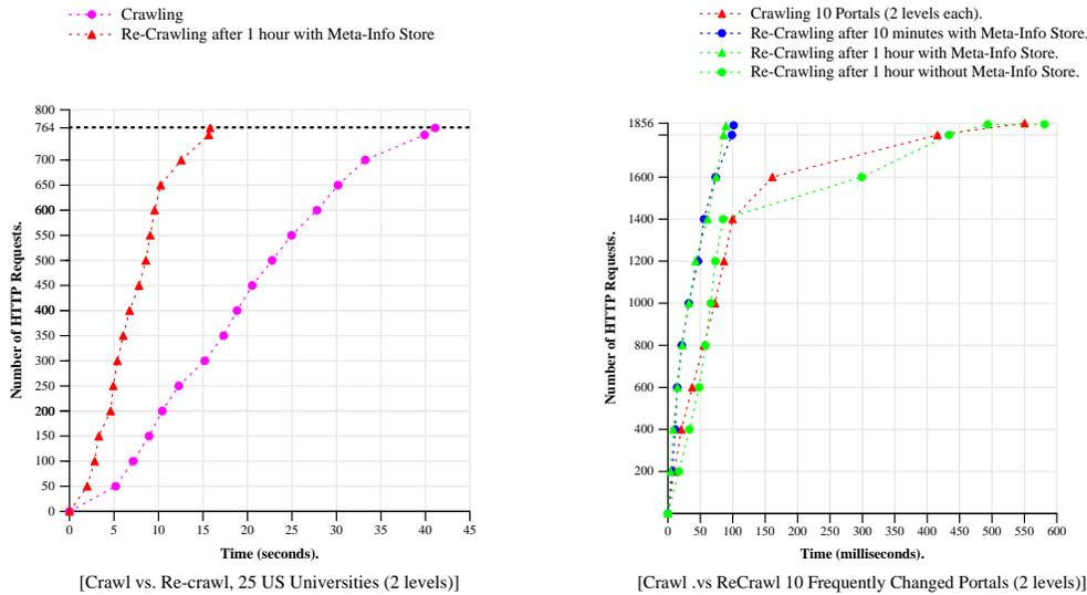
Figure 7: Crawling vs. re-crawling in WebRACE.
