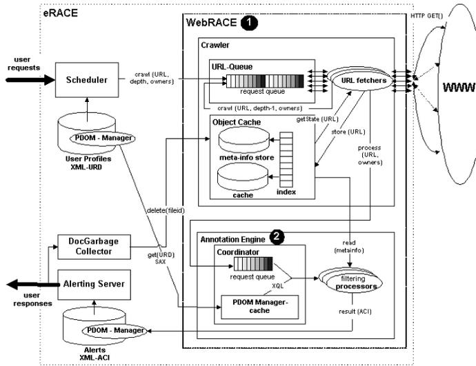
Figure 1: WebRACE System Architecture.
