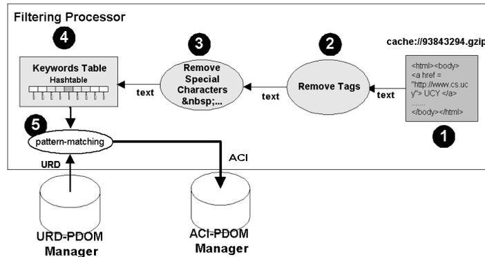
Figure 10: The Filtering Processor.
