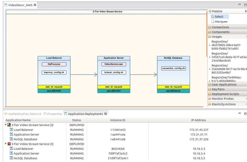
Fig. 4: Application Deployment on Amazon EC2 and Nephelae
