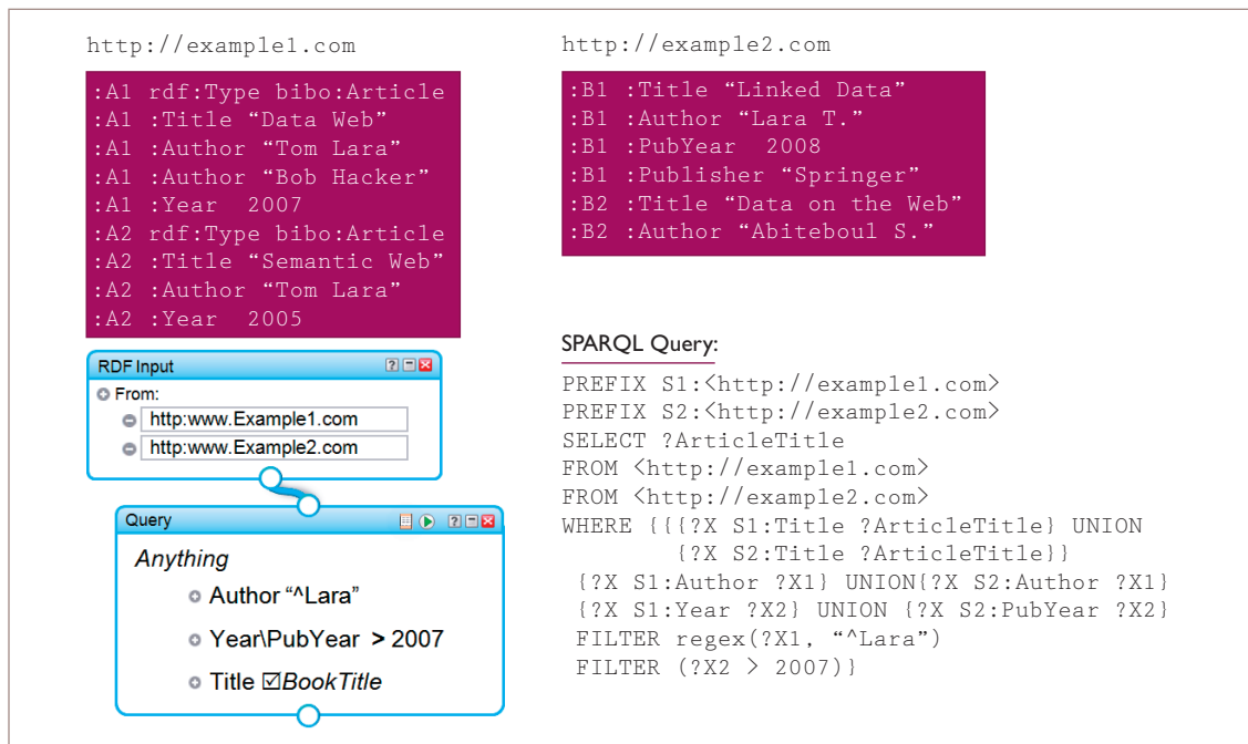
Figure 1. A query over two RDF data sources. Here, we’re trying to retrieve “anything written by Lara, published after 2007, and with a title.”
