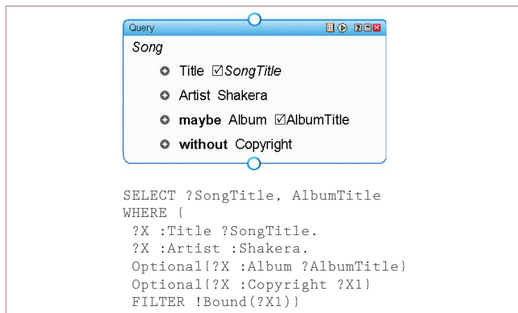
Figure 3. A MashQL query and its mapping into SPARQL. The query retrieves everything that has a title and artist, maybe has an album, and doesn't have a copyright.
