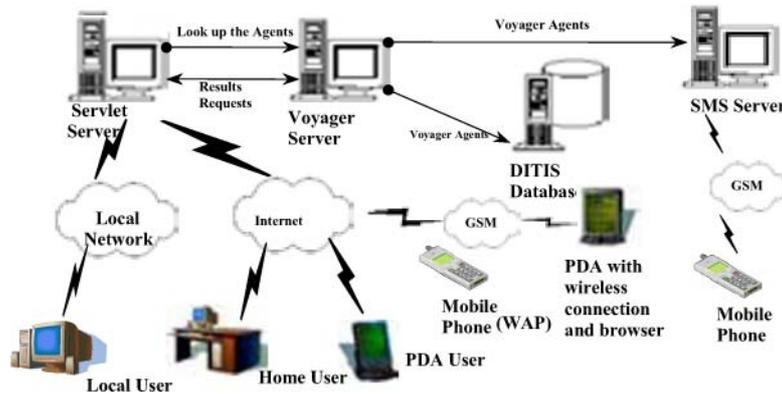
Figure 8. Schematic of DITIS system infrastructure
