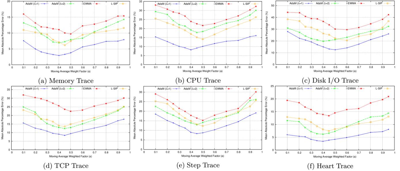
Fig. 5: Mean Absolute Percentage Error (MAPE) Comparison of Techniques Using a Moving Average Estimator
