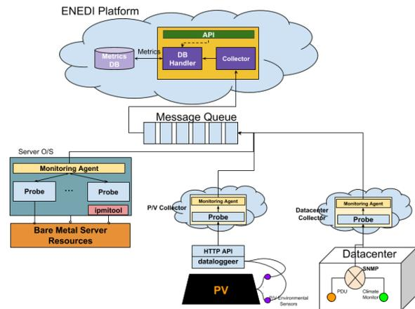
Fig. 2: ENEDI Monitoring System Architecture
