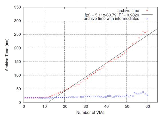
When archiving time is high, we can redirect monitoring metric traffic through Intermediate Monitoring Servers, allowing the monitoring system to scale
